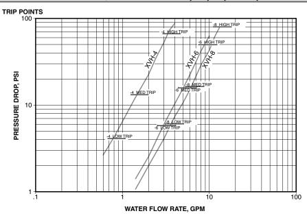
**Note**: XVH-4 is inlet/outlet size of '¼" XVH-6 is inlet/outlet size of '½", 6mm XVH-8 is inlet/outlet size of '½", 8mm
