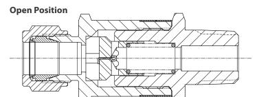
The spring holds the poppet in the open position during normal flow. When flow increases to the predetermined rate or trip point, the poppet will close.
