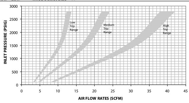
Air Flow – Low Inlet/Outlet Sizes = 3/8", 6mm
